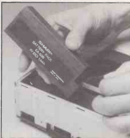
A rechargeable battery pack fits into a slot as the back of the casing.
