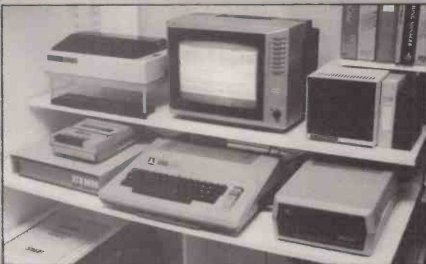
Atari 800 setup with Epson dot-matrix printer; ATR-8000 64K Z-80 expansion running 80-column CP/M 2.2, £399 from Tollgate; connected to a standard 5.25in. drive, £200 to £250.
