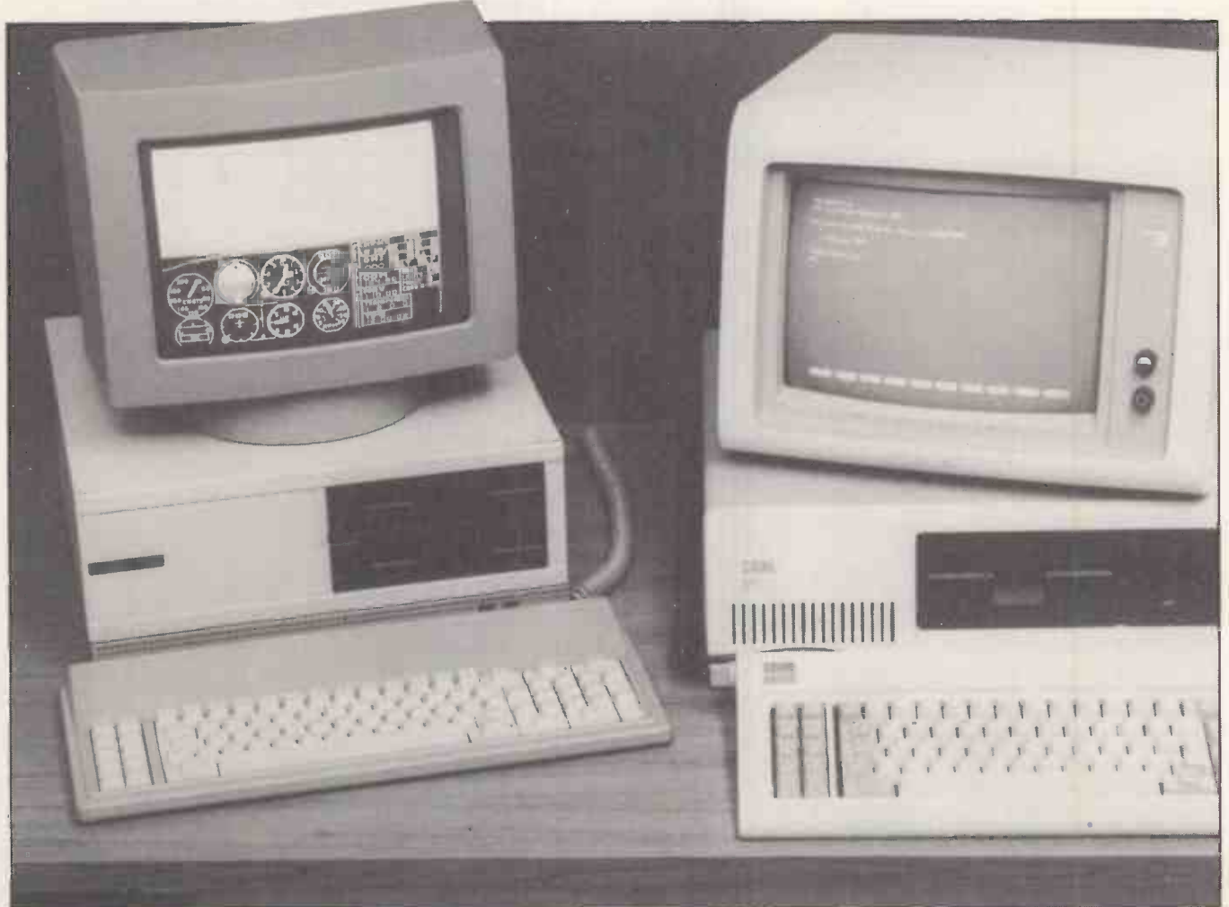
The M-24 offers full compatibility with the IBM PC XT (right) but is housed in a smaller, neater box.
