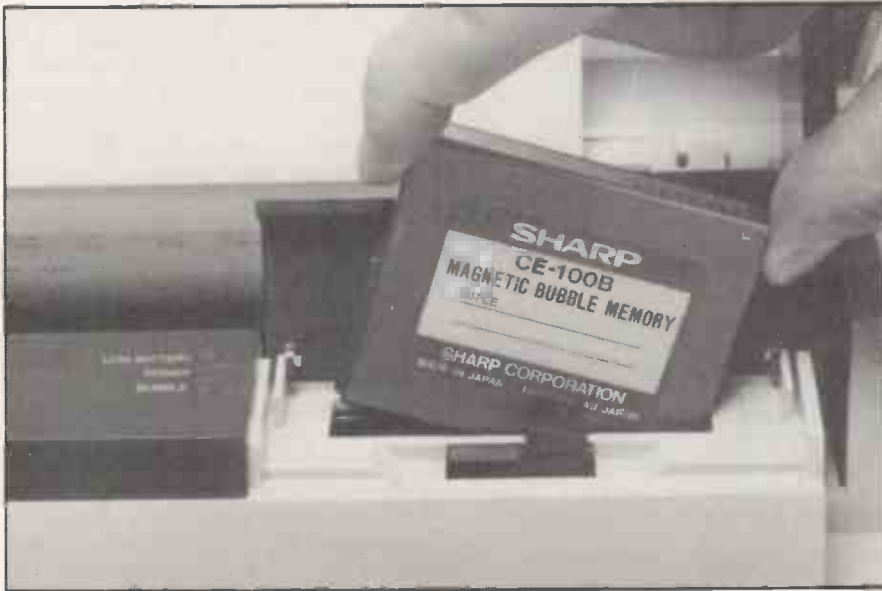
Below: The PC-5000 uses bubble memory for compact, lightweight mass storage.
